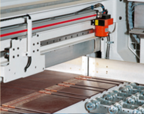
In use: The absolute measuring SGW wire-actuated transducer in a horizontal circular saw.
